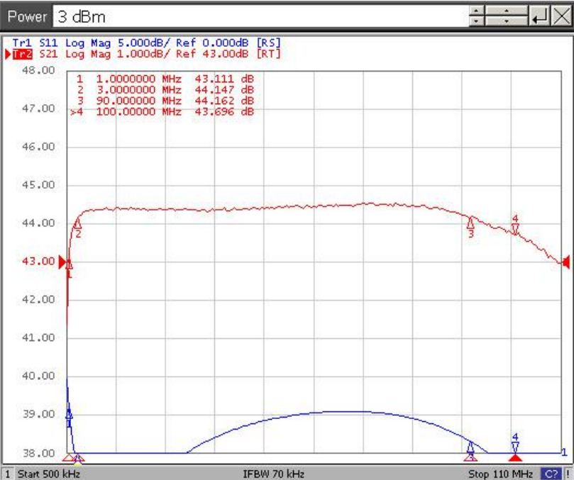
Frequency Response Curve @ 50 Watts Output
