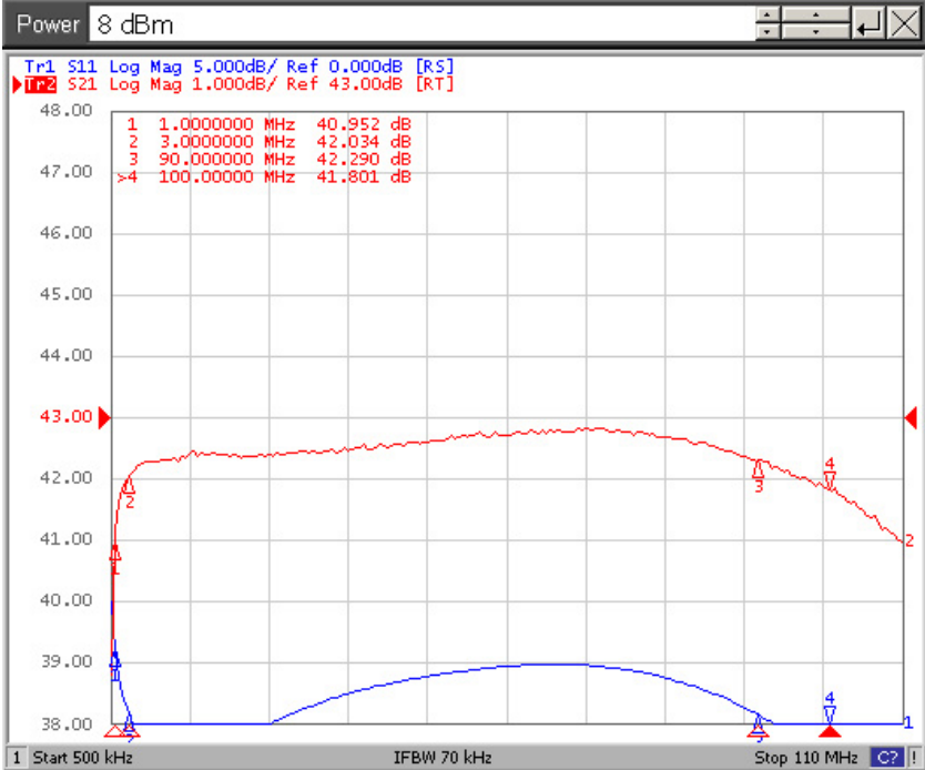
Frequency Response Curve @ 100 Watt Output
