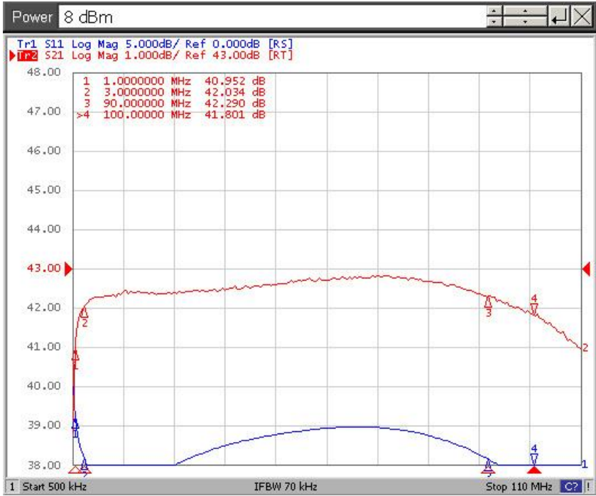
Frequency Response Curve @ 100 Watt Output
