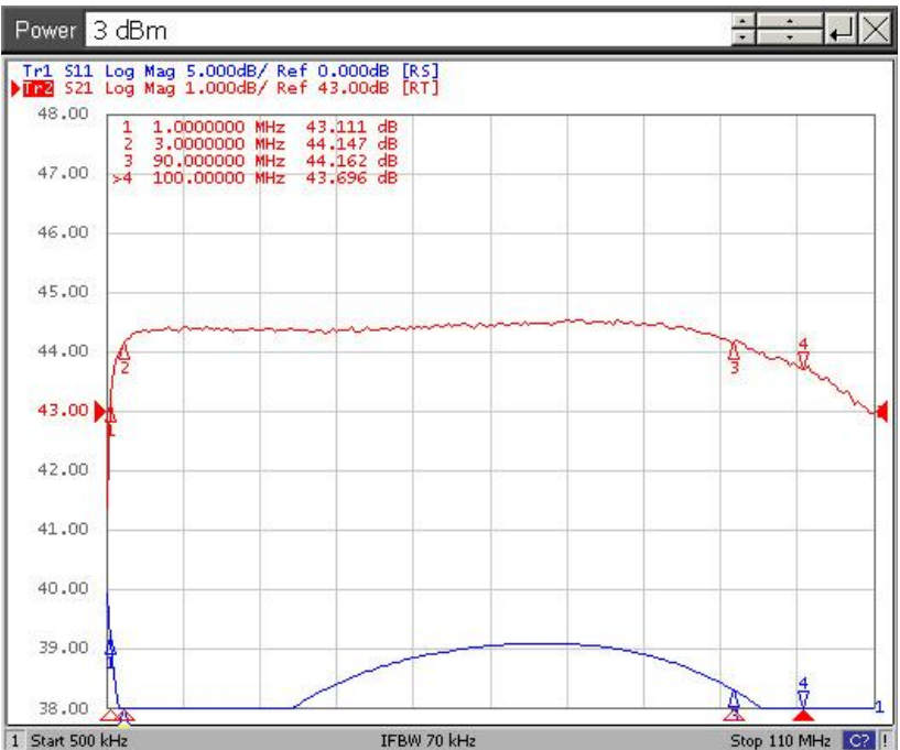
Frequency Response Curve @ 50 Watt Output
